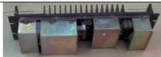
Unit with rear cover removed showing mechanical bracing of major components
