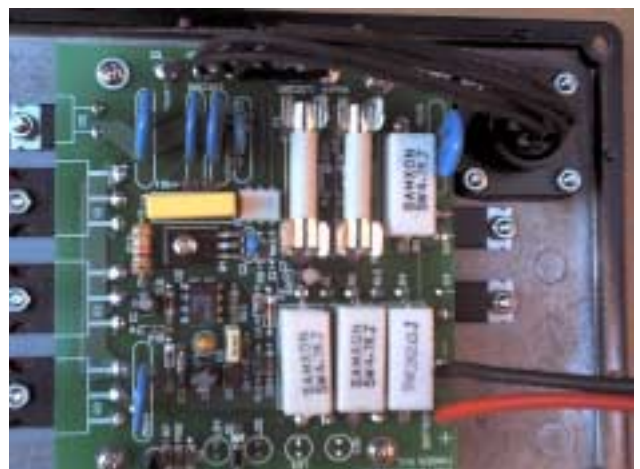
HRC Fuses and Panel Connector (components both sides of PCB)
