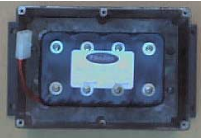
NiCd battery with integral shock mounts
